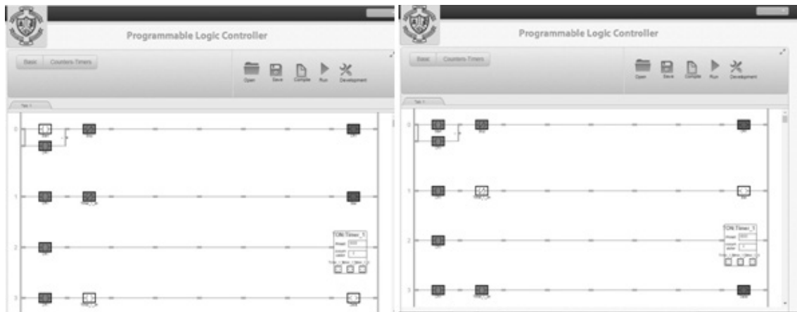
Figure 2. Implementation of PLC programming in VI lab
