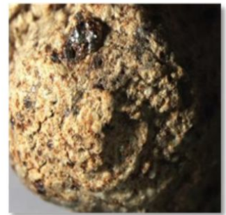
Figure-4 Microstructure of sintered flyash lightweight aggregate (10 \mu m and 1.5x)
