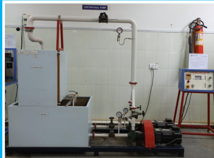
Centrifugal Pump Setup
