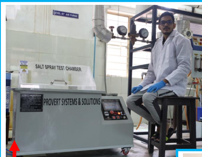
Ahmed is testing stability of composites in simulated ocean environment
