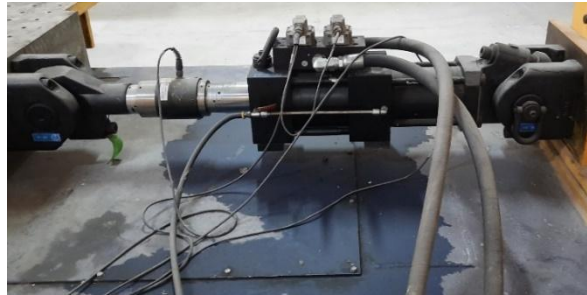
MTS ACTUATOR 250KN CAPACITY WITH HPU (TWO HOSE) AND CONTROLLER
