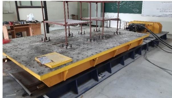
SHAKE TABLE (2m × 3m), 12 TON CAPACITY
