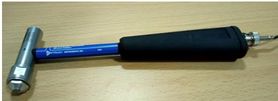
IMPULSE HAMMER WITH LOAD CELL TO RECORD IMPACT FORCE
