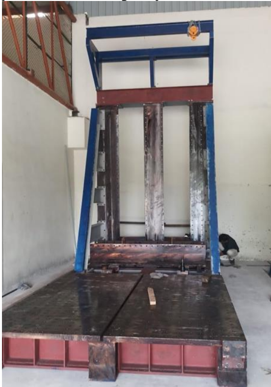
Horizontal Load test Rig (Static and Dynamic) 250kN capacity
