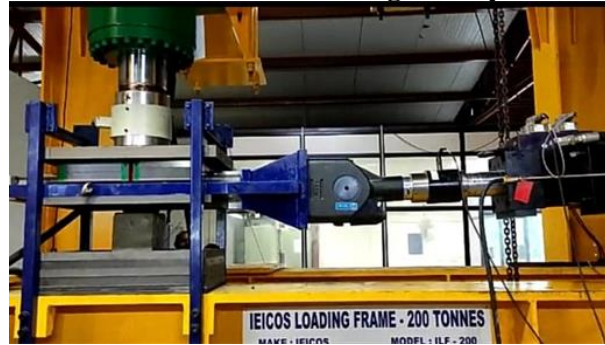
Base Isolator Testing facility
