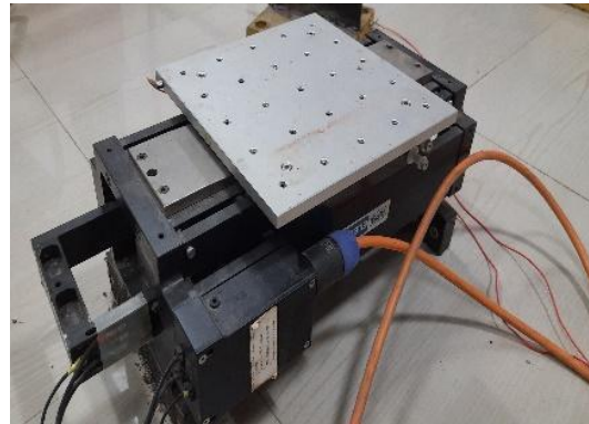
MINI SHAKE TABLE WITH ADDED MASS ASSEMBLY FOR VERTICAL AND HORIZONTAL TESTS AT FIELD
