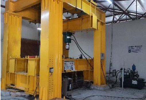
HEAVY LOADING FRAME 200 TON CAPACITY
