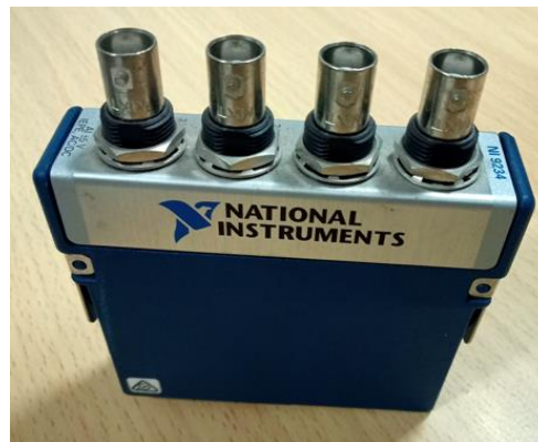
NI 9234 DAQ SYSTEM WITH LabVIEW SOFTWARE FOR SIGNAL RECORDING AND POST PROCESSING
