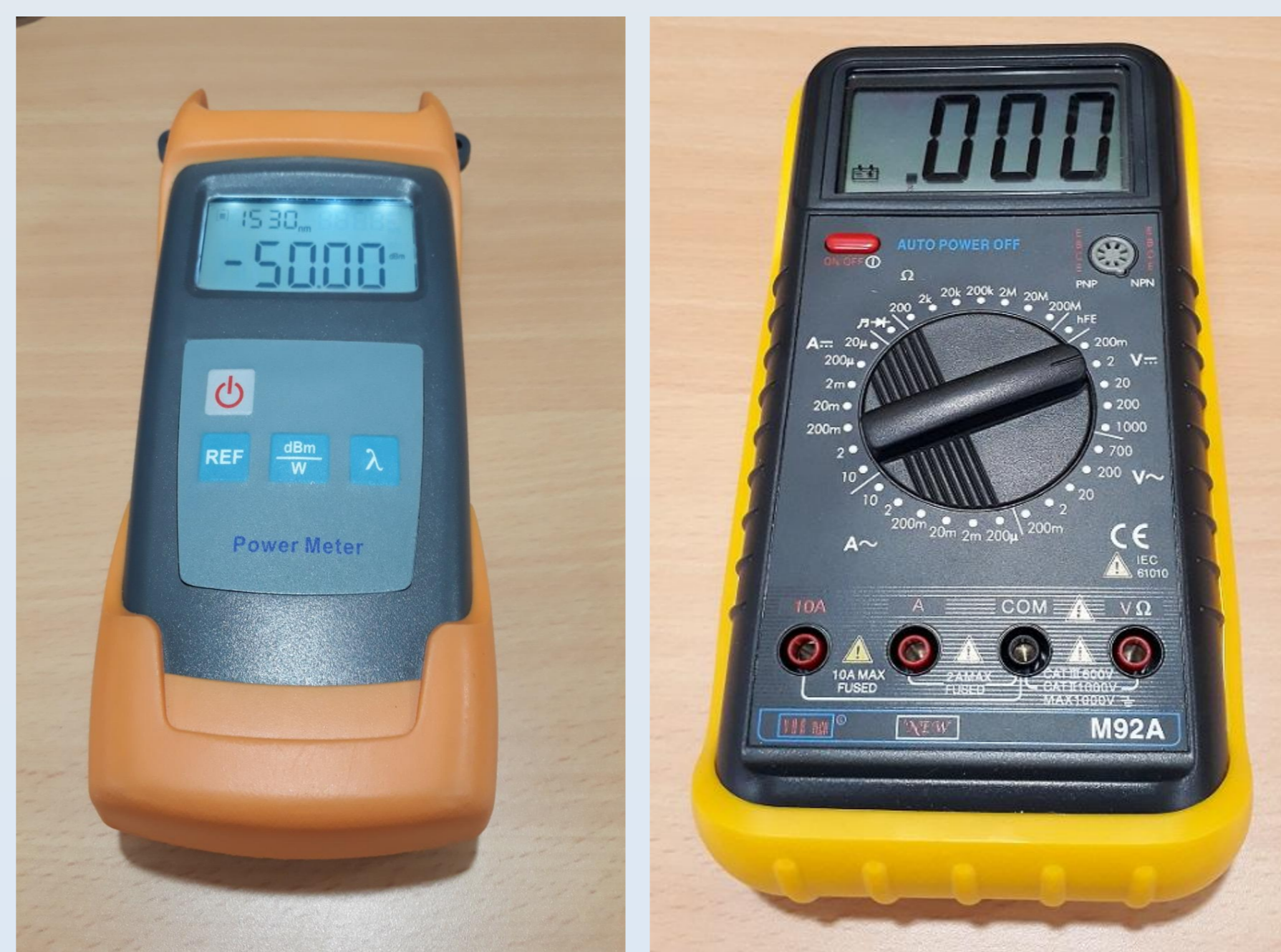
Power Meter Digital Multimeter
