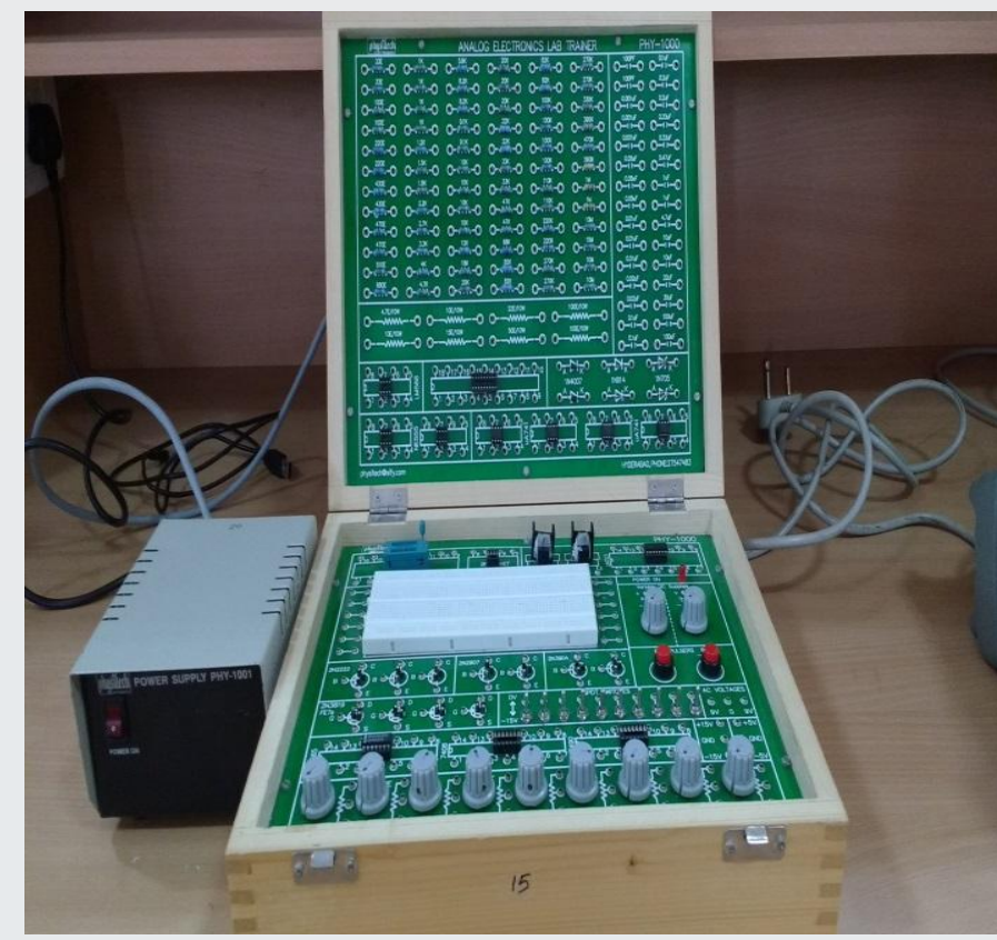
Analog Electronics Lab Trainer kit
